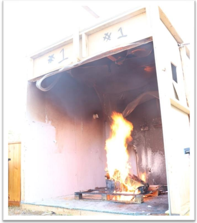
Figure 2: Plastic melting as fire grows. Time marked.
