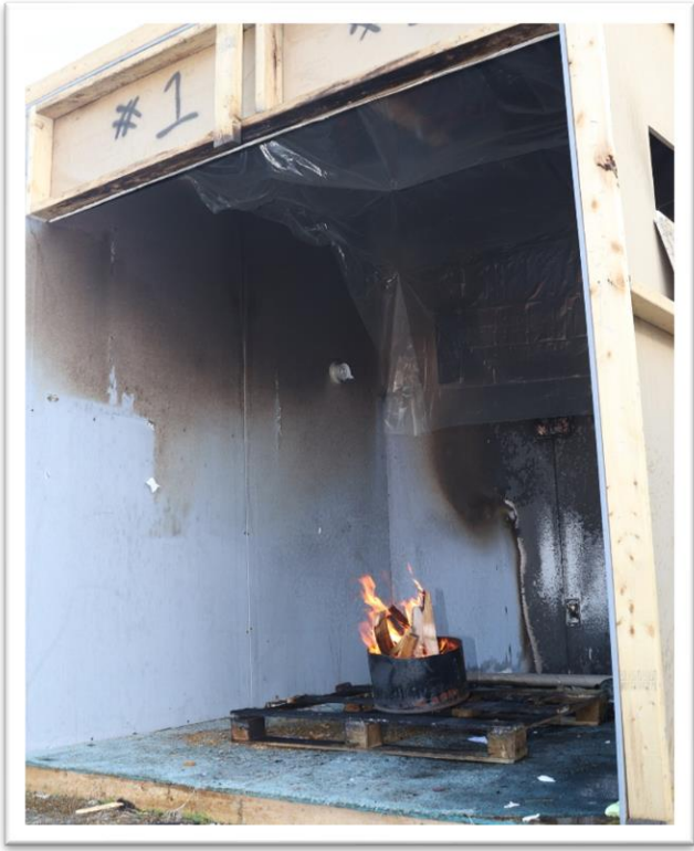
Figure 1: Sprinkler head blocked by plastic. Fire set.
