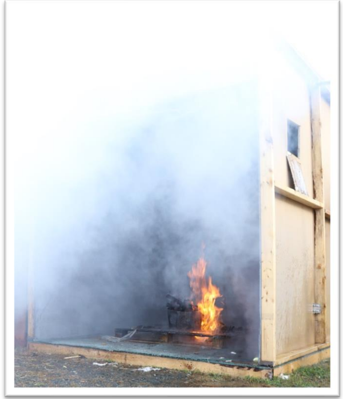
Figure 4: Fire extinguishing by sprinkler
