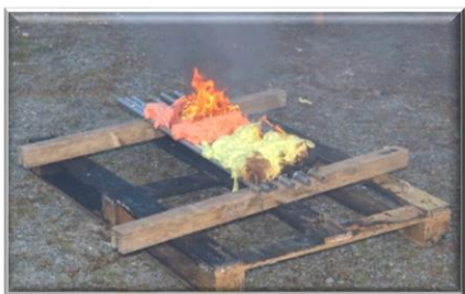
Above: Setting up burn cell tests, training and testing fire blocking consumer product claims October 2022.
