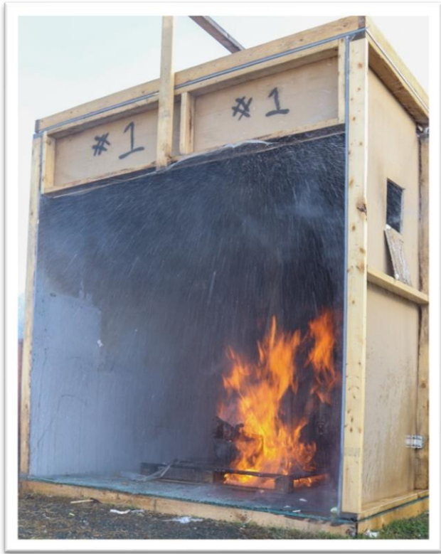
Figure 3: Sprinkler activated. Time marked.
